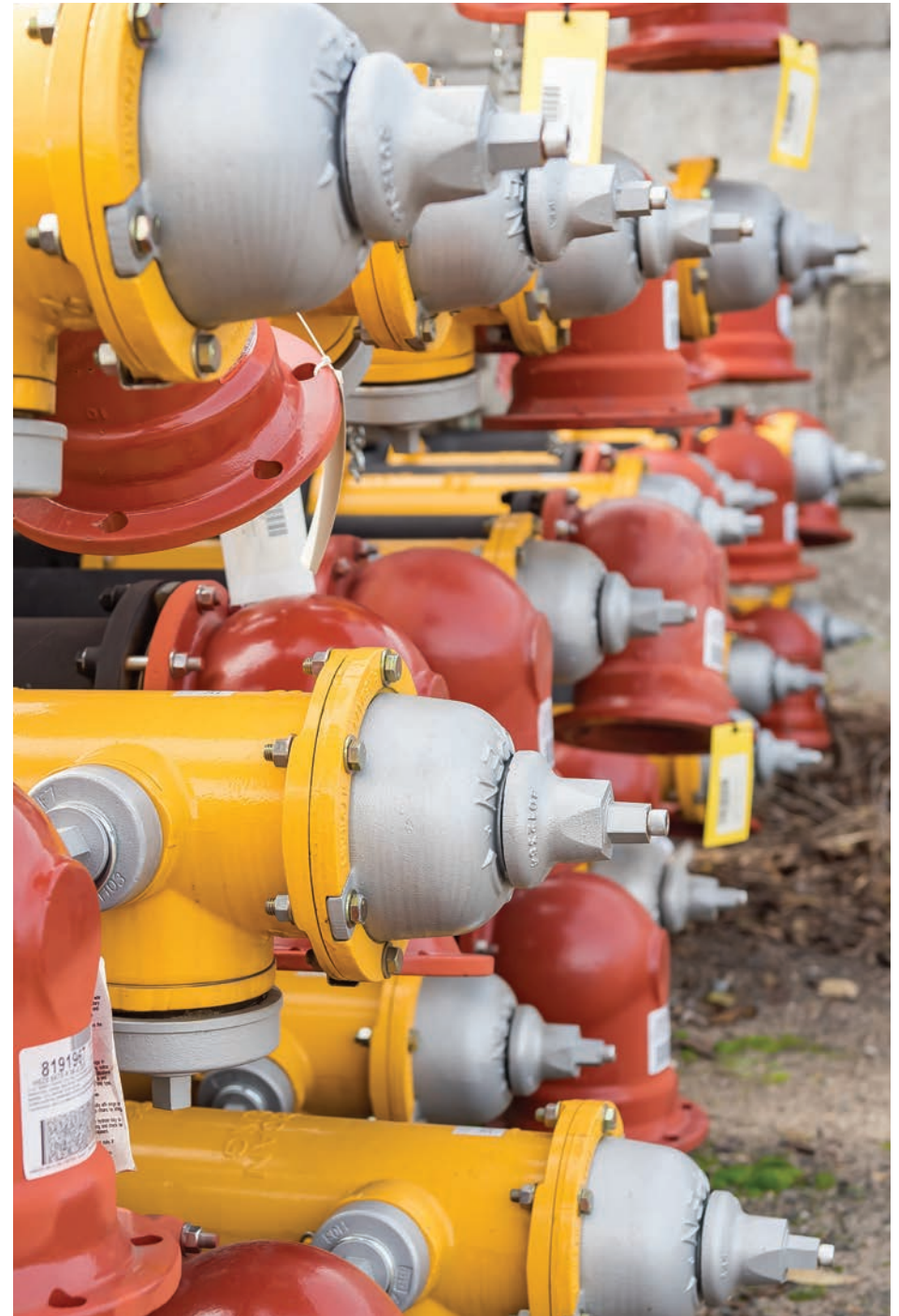
New fire hydrants.
