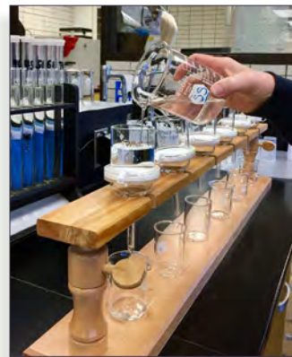
Water is filtered before being tested for organics
