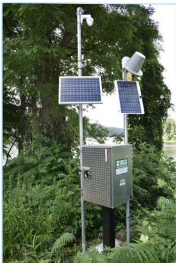
At left: A new river gauge was installed near the border of Vermont in Northfield, Massachusetts as part of a new nitrogen sampling program on the Connecticut River supported by the Commission, MassDEP, and the U.S. Geological Survey.
