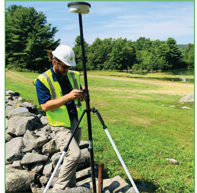
Above: A Commission land steward uses a new high-accuracy GPS unit to identify property boundary lines.
